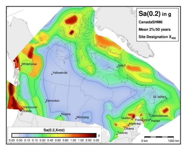
Map of the CanadaSHM6 short-period (0.2s) 5%-damped spectral acceleration at a 2% in 50 years probability of being exceeded for a Site Designation of X<sub>450</sub> (i.e., with a Vs30 of 450 m/s, equivalent to Site Class C in NBC 2015).
